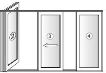
The second and subsequent panels slide up to the first panel and click into place.
