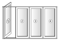
The first panel is hinged and can be on either side of the opening.
